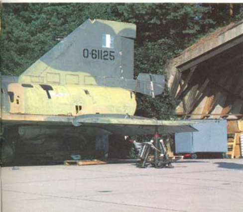
An ex-Greek Air Force F-102A showing the telltale signs of a battle damage repair bird. Shortly after this photo was taken, the aircraft was completely rebuilt and sprayed glossy grey. An ex-Greek F-84F in nearly mint condition received the same treatment
